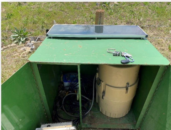
Figure 10. General view of the ISCO 3700 Portable Sampler located at the downgradient end of the ditch.
